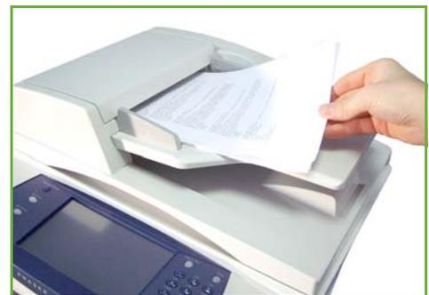
**i** Up to 100 sheets of 20 lb (80 g/m<sup>2</sup>) bond paper can be loaded. Weight ranges from 12.5 lb to 28 lb (50 - 120 g/m<sup>2</sup>) - refer to Machine Specifications in the Specifications chapter on page 204. for full Document Feeder Specifications.
