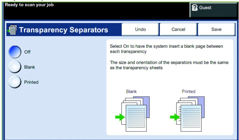
Select **Blank** to have the system insert a blank page between each transparency, or select **Printed** to insert a printed page between each transparency. Then choose the appropriate transparency and separator stock.
