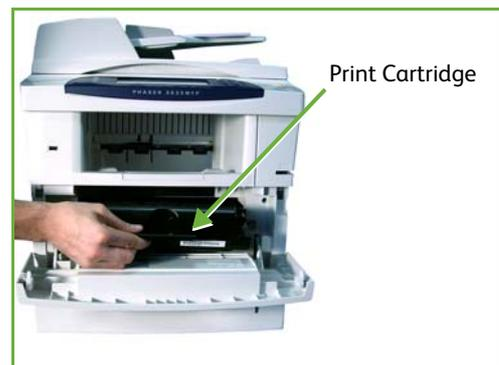
**i** If after fitting a new Print Cartridge the front door will not close, check that the Print Cartridge is positioned and latched correctly.
