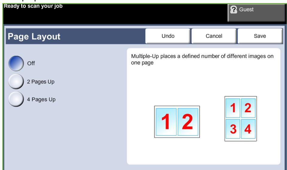
**NOTE:** Originals must be loaded in the document feeder when using this feature.
