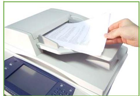
**i** Up to 100 sheets of 20 lb (75 g/m<sup>2</sup>) bond paper can be loaded. Weight ranges from 12.5 lb to 28 lb (50 - 120 g/m<sup>2</sup>) - refer to Machine Specifications in the Specifications chapter on page 204. for full Document Feeder Specifications.
