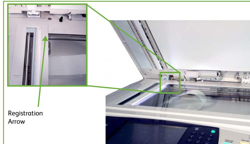
2. Place the document face down on the document glass, aligned with the tip of the registration arrow near the top left of the document glass.
