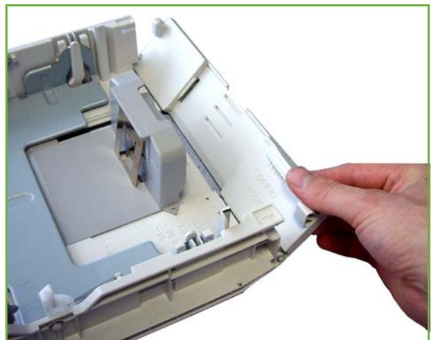
4. Move the guides so they just touch the paper stack. The guides must lightly touch the edge of the stack, neither too tight nor too loose.
