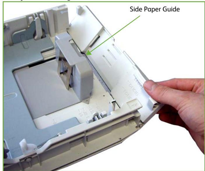
4. Fan the paper and insert it into the tray. If loading Letterhead, ensure the design is face-up and the top edge of the sheet is placed at the right side.
