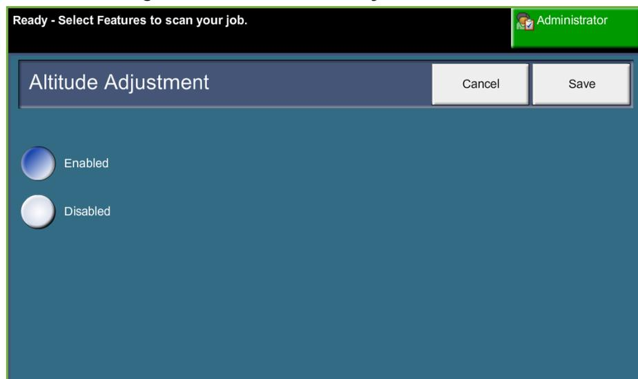
Setting the altitude enables the machine to operate effectively and maximises performance.
