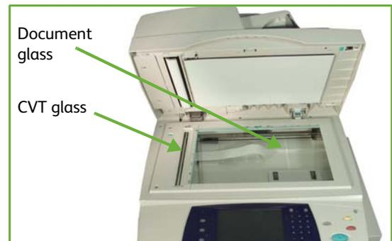
**NOTE:** Spots or marks on the glass will be reproduced on the prints when copying from the document glass. Spots on the Constant Velocity Transport Glass will show up as streaks on the prints when copying from the document feeder.
