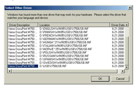
Scroll down to the selection named USB $\X750$ USB.INF (or X760USB.INF when installing M760) and click on it
