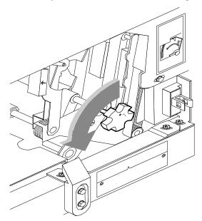
3. Push and hold the green handle to the left (in the direction of the arrow marked on it). Remove and discard any paper you find there.
