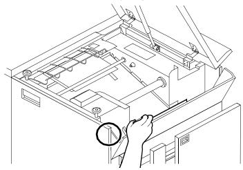
5. Remove only the set of pages leaving the stitcher/stacker at the right, and place it on the output in the stacker tray. Do not remove any other pages from this area.
