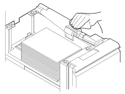
3. Latch the paper feeder assembly by pressing down on the bright green dot. Slide the paper tray completely back into the printer.
