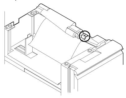
2. Lightly moisten a lint-free towel with film remover and thoroughly wipe the outside surface of the feed belt in the same direction as the ribs on the belt. (Wiping from side to side might pull the belt off its track.) Allow a few seconds for the film remover to evaporate.
