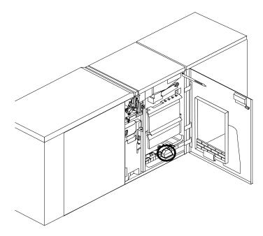
2. Lift the three green handles one by one. Each time you lift a handle, remove and discard any paper you find beneath the open section.
