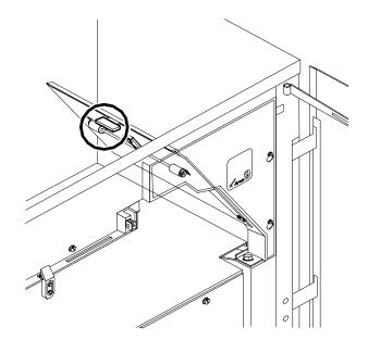
2. Pull the green handle down and to the left (in the direction of the arrow marked on it) to hold the assembly open while you remove and discard any paper you find in this area.
