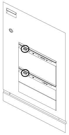
3. When the Ready To Open indicator is lit, pull the bar up and out to open the tray. Pull the tray all the way out for best results.
