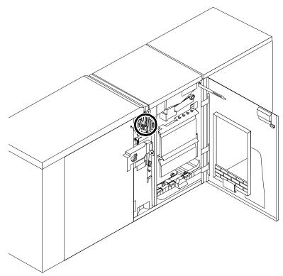
2. If paper is caught in the rollers between areas 4 and 5, first turn the green knob in the direction of the arrow marked on it. This ensures that the paper has completely moved into area 5, where you can remove it without tearing it.
