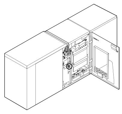
2. Push and hold the green handle to the right (in the direction of the arrow marked on it).
