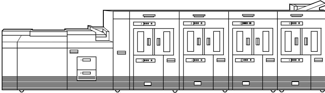
**Figure 1-10 Printer with inverter feeder/stacker + feeder/stacker + feeder/stacker + feeder/stacker**
