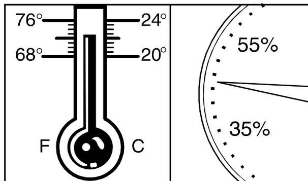
**Figure 4-2 Recommended temperature and humidity for paper storage**
