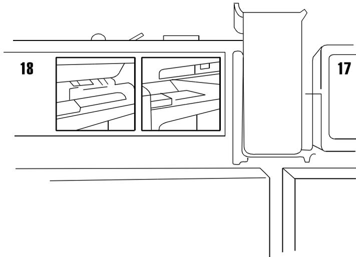
**Figure 5-1 Area jam clearance labels inside the printer**
