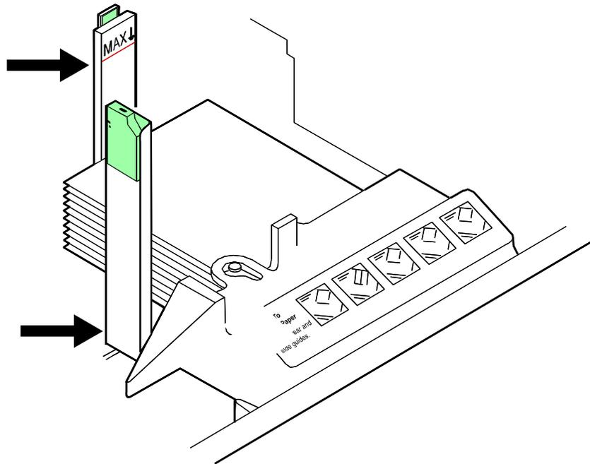
**Figure 2-7 Rear and side guides in trays 3, 4, 5, and 6**
