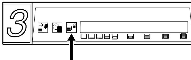
**Figure 5-22 If necessary, press Tray Unlock button**
