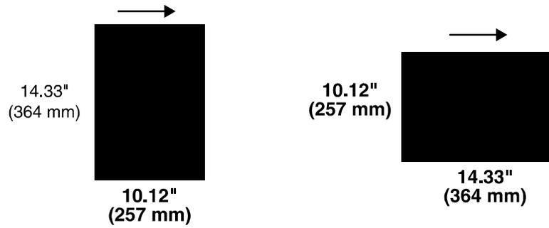
Figure 1-31 JIS B4 (257 by 364 mm) paper feeding (may be long or short edge feed)
