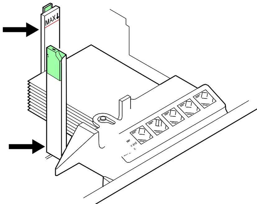
Figure 2-10 Press green dot on tray latch
