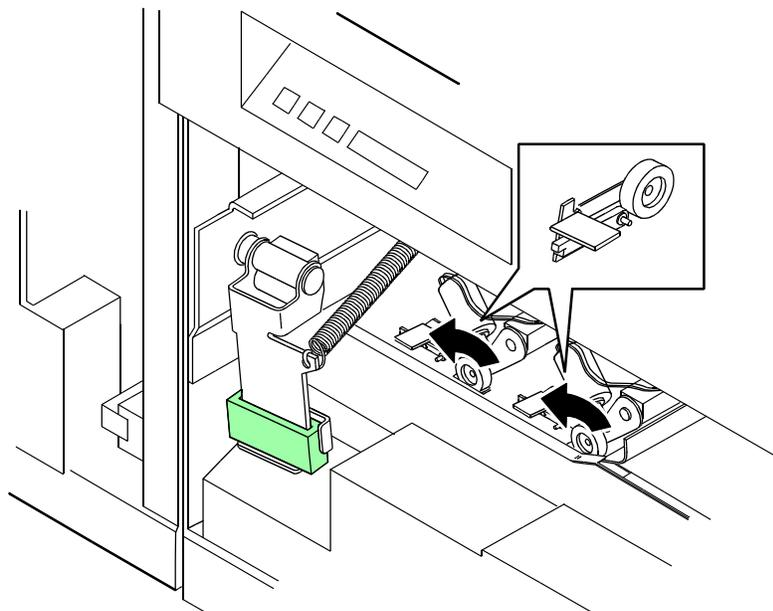
**Figure 2-1** Turning the registration transport roll levers
