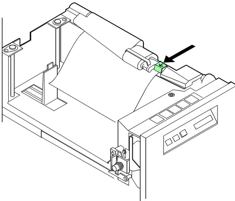
**Figure 5-25** If necessary, unlatch paper feeder assembly
