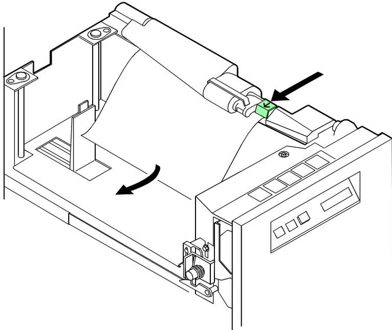
**Figure 5-23 Green lever to unlatch paper feeder assembly**
