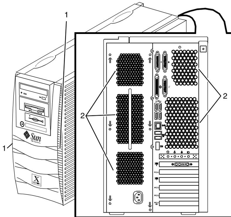
Figure 1-19 Sun Blade 1000/2000 fan/vent locations to keep clear
