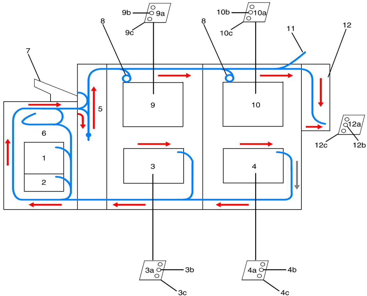
**Figure 1-13 Route of paper through the printer**
