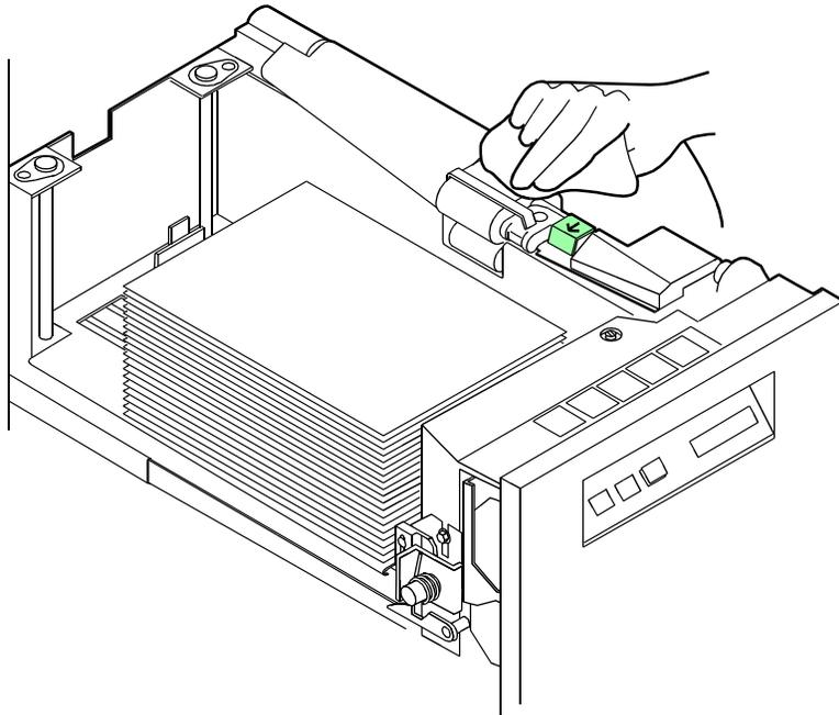
**Figure 5-26 Wipe outside surface of feed belt**
