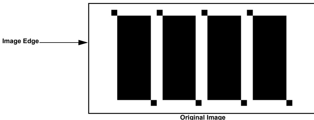
Register allows you to define the position of the image content (the black pixels). When you register the above image, you are moving the black pixels of the image. The size of the image does not change.
