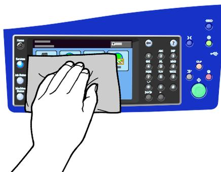
2. Use a lightly dampened cloth to clean the outside of the document feeder, output trays, paper trays, and outside areas of your printer.
