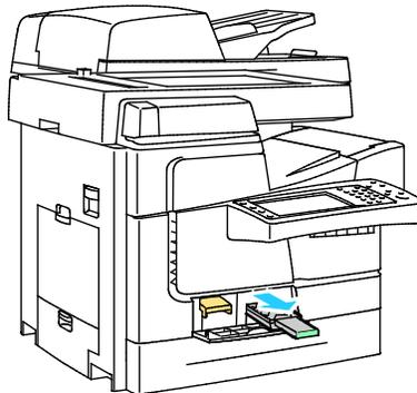
3. Empty the waste tray in a waste container. Twist the waste tray slightly to dislodge the waste ink. The ink is non-toxic and can be discarded as normal office waste.
