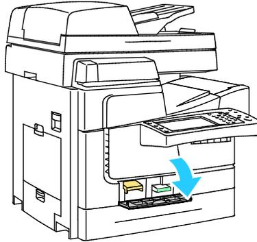
2. Remove the waste tray from the printer.
