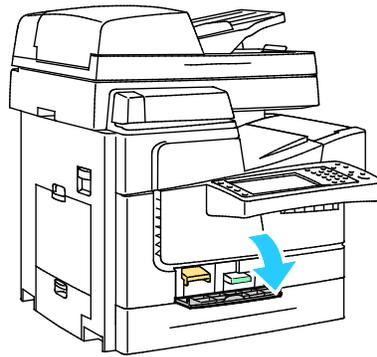
2. Remove the cleaning unit and place it in a plastic bag for storage.
