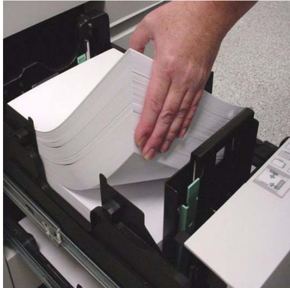
Figure 2-5. Fanning the lead edge
